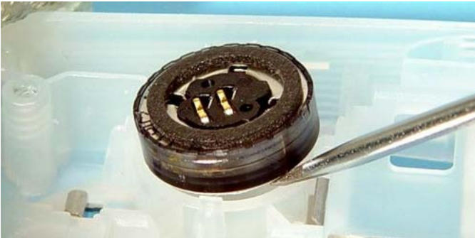
The SALT Speaker is taped to the D-Cover and can be removed with a straight bladed screwdriver.
